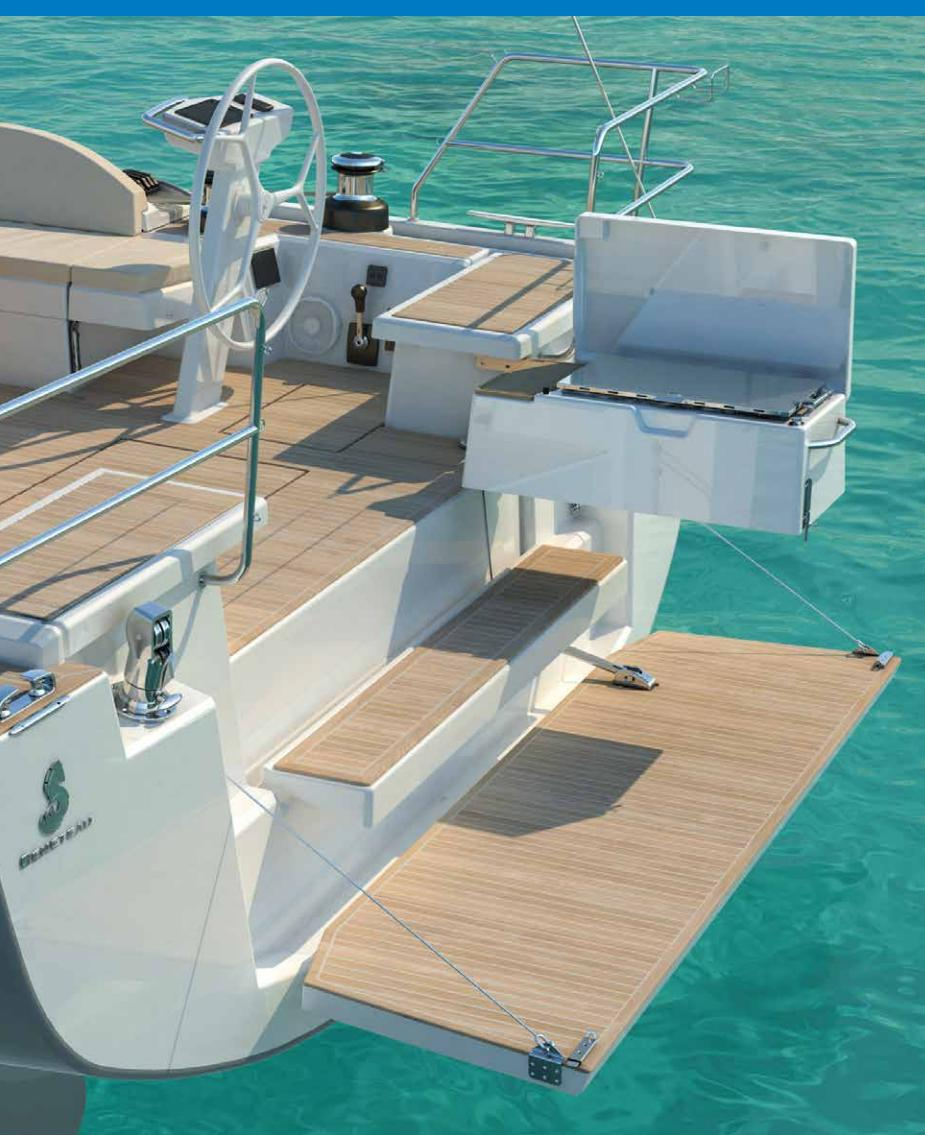
The huge cockpit table, retractable davits and the plancha grill built into the aft bench reveal a **practical** and **cleverly equipped** cruising yacht.
