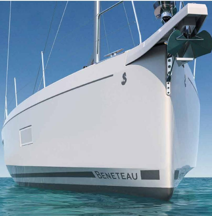
Originating from a drawing by Olivier Racoupeau, the stepped hull extends over a third of the hull from the bow and marks a major development. Apart from her attractive lines, this choice **increases the amount of space inside** for fittings unheard of on a boat this size.
