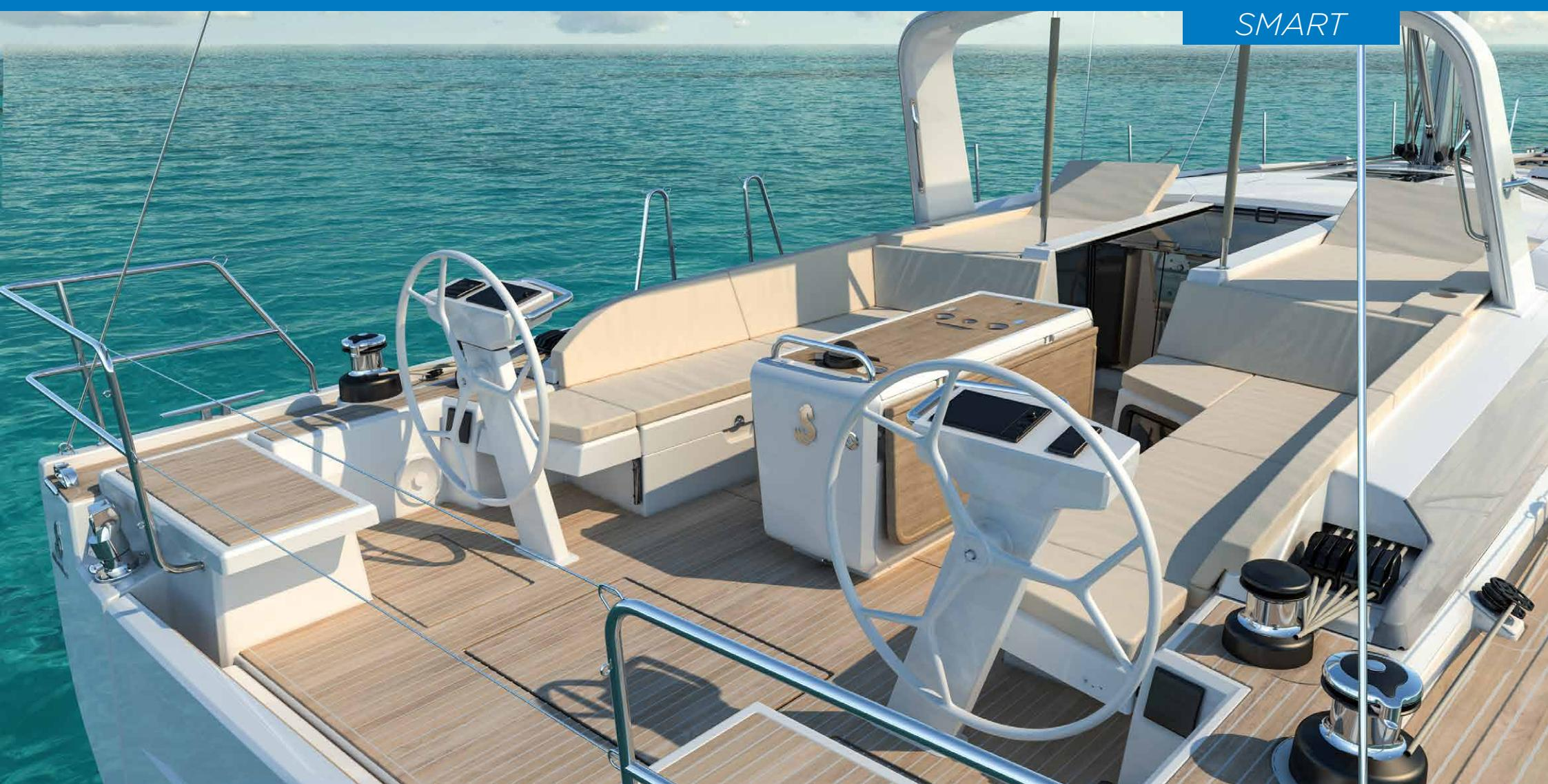
**Safety and comfort** come first at the two steering stations: removable foot straps, the position of the winches and the steering consoles are all part of her well-designed ergonomics.
